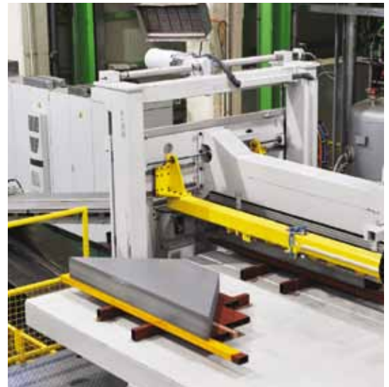
- AUTO CORE CUTTING MACHINE (CUT TO LENGTH)
